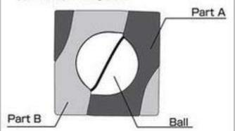
Keep Part A and lower ball half from moving, then twist the Part B and upper ball half together.
