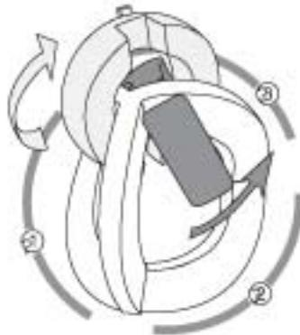
Angle ring A towards position ③ while raising it at the location where it is almost fitted into the frame.
